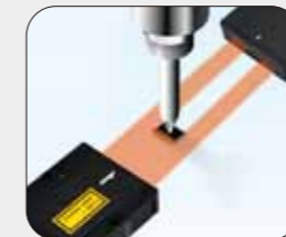
Locating a small IC chip held by a vacuum pickup
