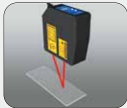
Monitoring warping sagging of glass plate
